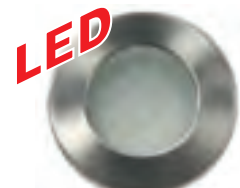
NEW LED42FSRMN LED Fixed recessed or surface mount with surround supplied. Led downlight of superb quality with 42 LED's for high output. Connect to 12volt DC. 2.5w Size 70mm Ø x 17mm recessed or 32mm High surface mounted.
