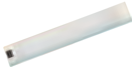
Slim dual strip light with 2 x 8w fluorescent tubes & 3 way switch, Size L 380 x W 65 x H 30mm. White ABS casing milky PS lens. L2208DW Slim dual strip light
