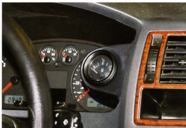
I also wanted a gauge rather than just a low-level warning, so fitted one, purchased from DieselVeg, on the side of the recess.
