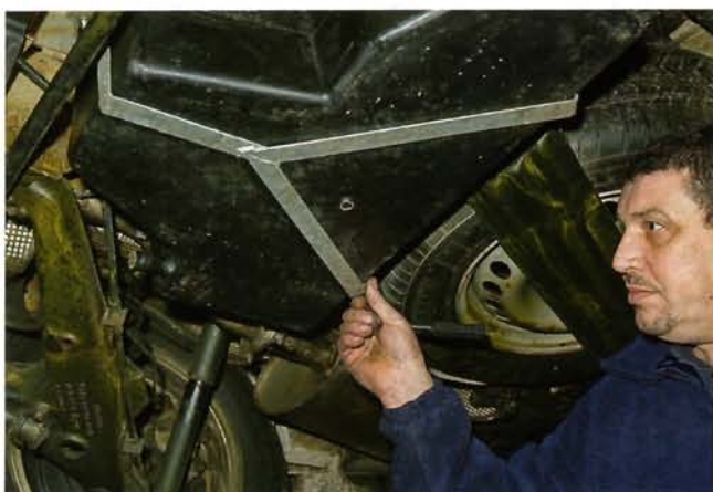
The CAK tank comes with its own mounting bracket. I had mine galvanised.
