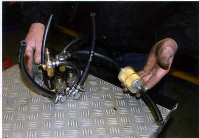
Under-bonnet solenoids switch between diesel fuel and vegetable oil, as required. Hoses are easier to connect before fitting. Extra filters are supplied.
