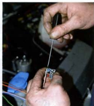
The wiring supplied is connected to solenoids and switches according to the comprehensive instructions and wiring diagrams supplied with each kit.
