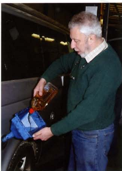
Rather than get involved in recycling dirty used cooking oil, the simplest approach is to use fresh cooking oil from the supermarket, in 1-litre containers.
